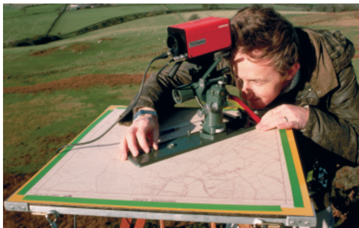
Figure 1 Cartographers in the field use technology to enhance the precision of their measurements. Electronic devices can be used to measure the distance between an observer and a distant point with a high degree of accuracy.
