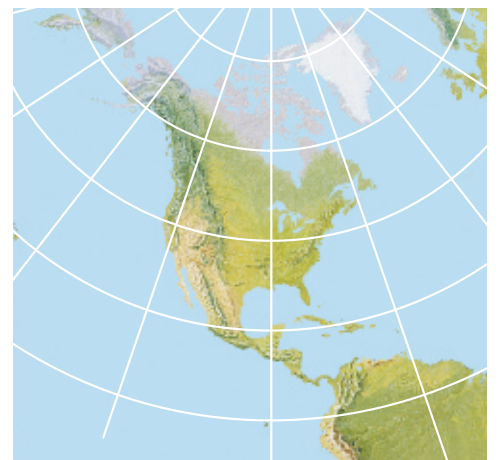
Figure 4 A light at the center of a transparent globe would project lines on a paper cone (left) that would produce a conic projection (right).
